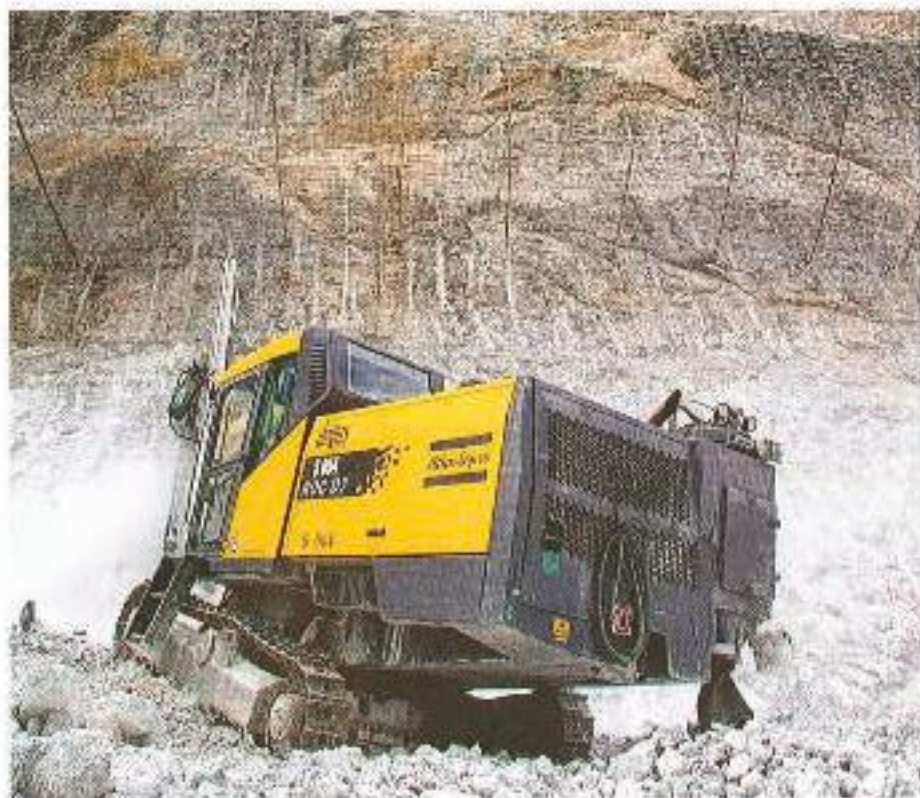
Bench test: The modified ROC D7 managed to exceed the drill plan specifications that required a maximum 40 cm wide shelf.
